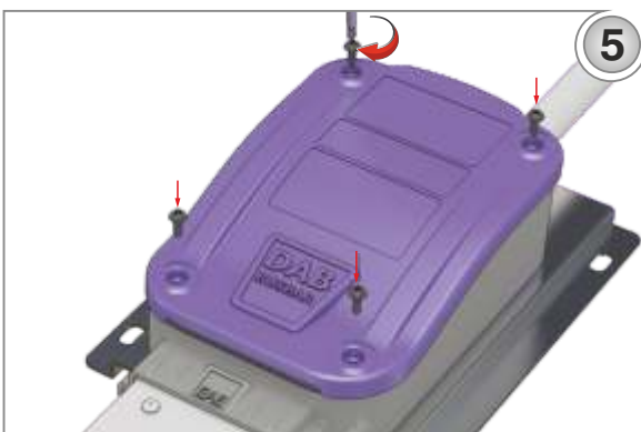
5- Refit the Feed Box cover by replacing the screws as shown. Be sure to use "U" support for the installation.
